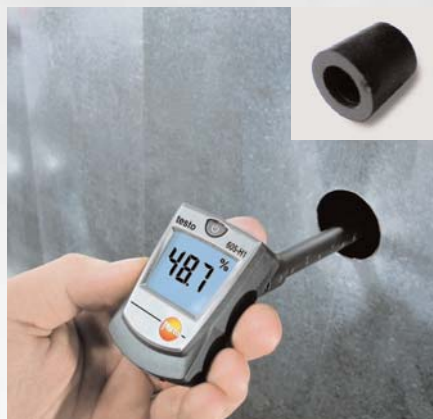
The testo 605-H1 and testo 405 have a duct fixture which guarantees that the measuring instrument is securely fixed in the duct.
